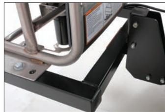
The mounting kit is custom designed to fit on the Classen SA30 stand-on aerator for simple and accurate installation. No cutting, drilling or fabrication is necessary to secure the attachment.
